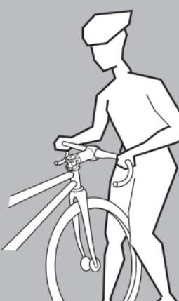
After installing the stem, check that the cable housings do not bind. Check by turning the handlebar until the grip hits the frame. If the housings bind, replace with longer ones.
